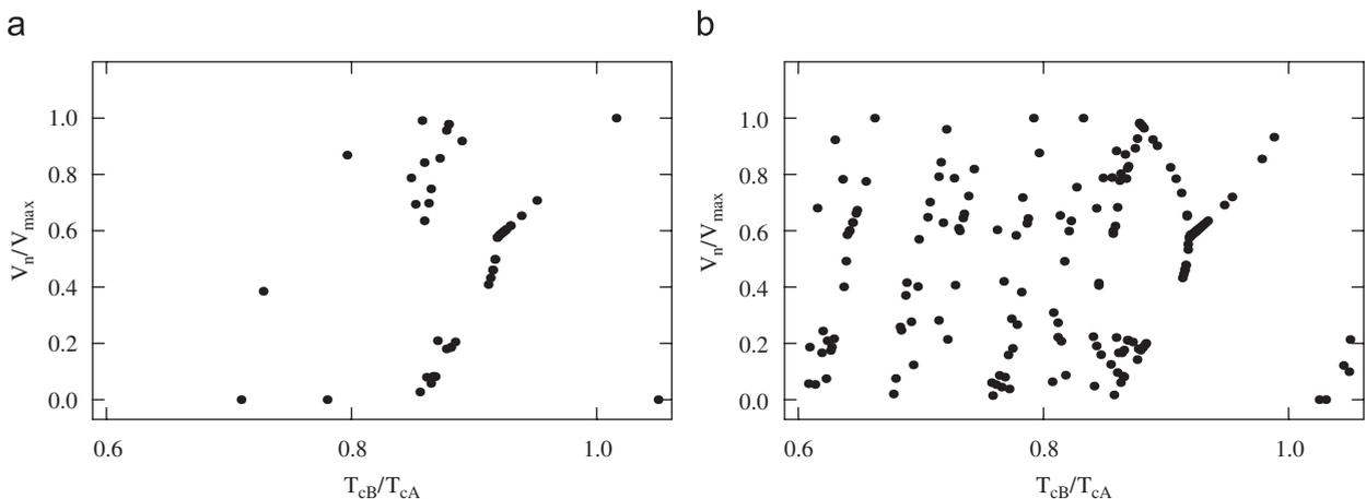
Fig. 4. The bifurcation diagram for the speed against  $T_{c,B}/T_{c,A}$  for two different values of  $x_{\text{tol}}$ , (a)  $x_{\text{tol}} = L_A/2$  (low risk of collision) and (b)  $x_{\text{tol}} = L_A/6$  (high risk). The other parameters are as in Fig. 3:  $L_A = 200 \text{ m}$ ,  $a_+ = 2 \text{ m/s}^2$ ,  $a_- = 6 \text{ m/s}^2$ . The transient has been removed.
