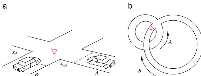
Fig. 1. (a) A sketch of the intersection to be studied: *B* is the mobile approaching the yield sign; *A* has preference to pass.  $x_d$  is the distance at which *B* must make a decision to stop or not.  $x_{tol}$  should be such that collisions are always avoided [see Eq. (1)]. (b) The roads are made to intersect at a periodic number of points.
