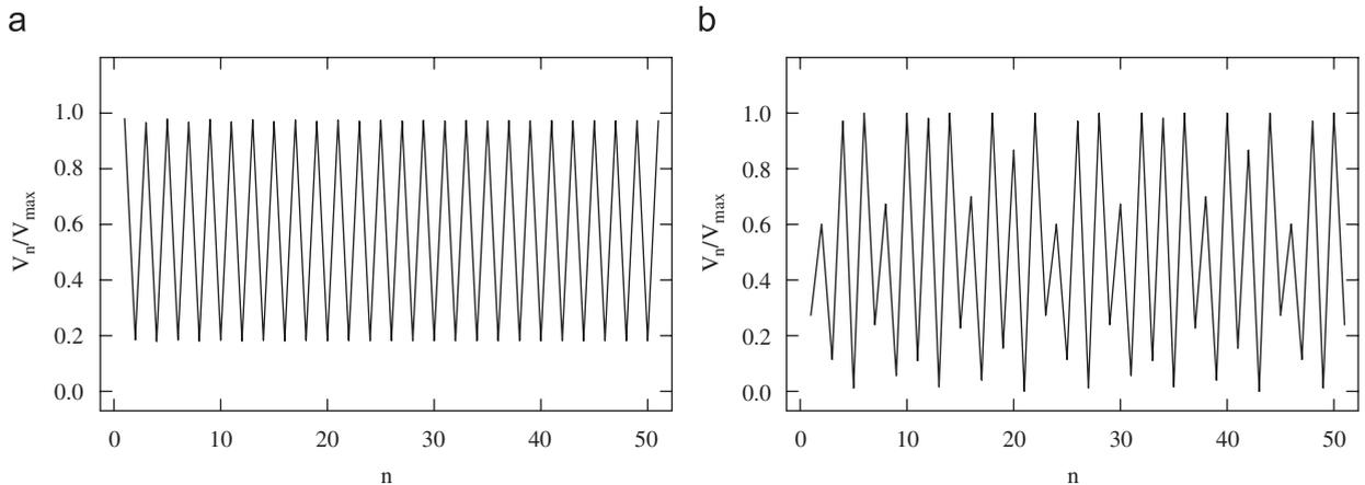
Fig. 3. The iterated map for the speed  $v_n$  at the  $n$ th crossing point, for: (a)  $T_{c,B}/T_{c,A} = 0.88$  and (b)  $T_{c,B}/T_{c,A} = 0.856$ , for  $x_{\text{tol}} = L_A/2$ ,  $L_A = 200 \text{ m}$ ,  $a_+ = 2 \text{ m/s}^2$ , and  $a_- = 6 \text{ m/s}^2$ . The transient has been removed.
